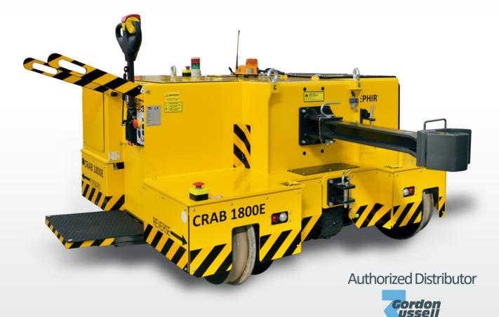
MAXIMUM DRAWBAR PULL: 4,045 lbf (18 kN) WEIGHT: 8,820 lbs (4.4 US t) DIMENSIONS LxWxH: 85.8"x72.0"x61.0" (2180 mm x 1830 mm x 1550 mm) UNLOADED RAIL SPEED: 3.1 mph (5 km/h) RAIL SPEED AT MAX LOAD: 1.2 mph (2 km/h) STANDARD GAUGE: 56.5" (1435 mm)
