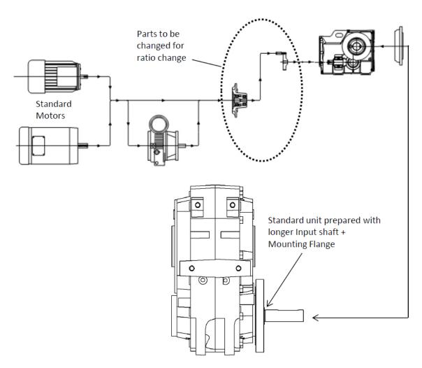
Multi-use kits: Utilising common components between types & Ratios. Full range of features available for all the mounting requirements from series J and series K.
