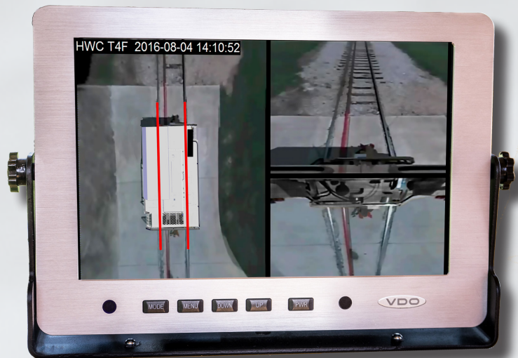
Display screen with operator selected tri-view. Left screen shows machine on rails, while right split screen shows front and back couplers.
