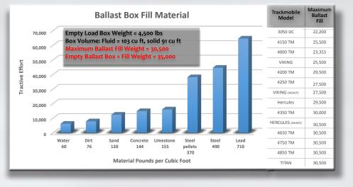
Equipped with an AAR profile coupler that can be extended or retracted, the Ballast Box can fit most Trackmobile railcar movers. Use the Trackmobile Model list to the right of the Fill Material chart to determine the maximum amount of fill that can be used in the Ballast Box for your specific Trackmobile model.
