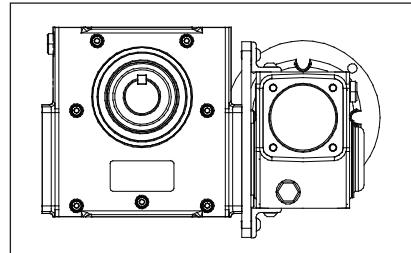
Motor Ready Double Reduction Reducer Unit
