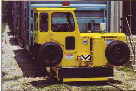
This single coupler vehicle is a real workhorse capable of moving seventeen 100 ton cars.
