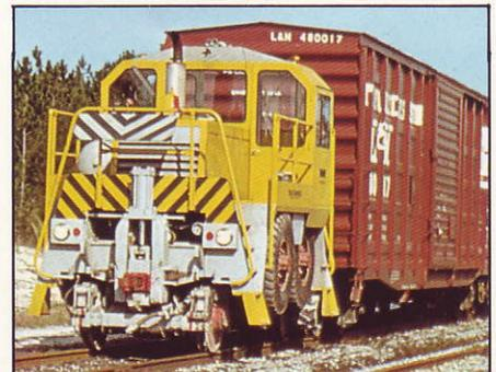
Capable of moving fifty 100 ton cars and a 30 MPH rail speed, the 11TM is built for speed and power for long hauls as well as spotting and switching operations.
