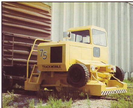
Here's the power and economy of a double coupler TRACKMOBILE, capable of moving thirty two 100 ton cars.
