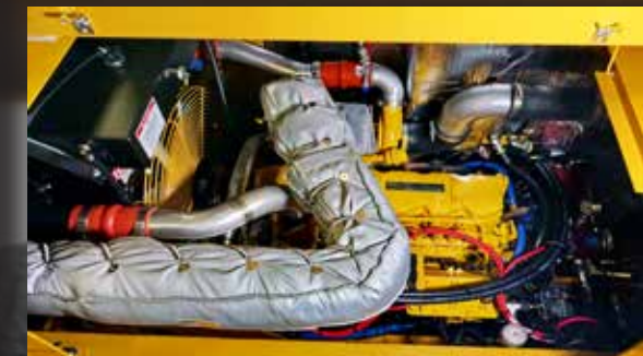
QSB-6.7 Liter Cummins Electronic Turbocharged Diesel Engine
