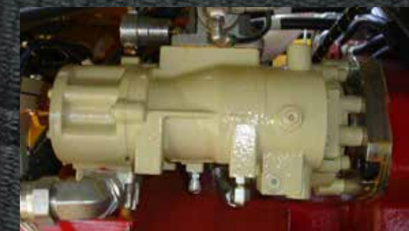
100 CFM Rotary Screw Air Compressor offers 100% duty cycle
